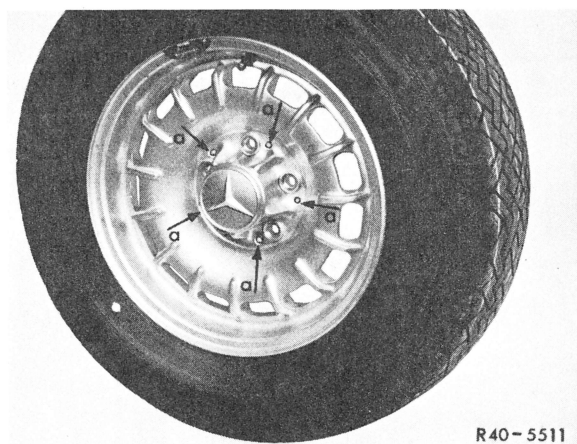
Fig. 1 a Receiving holes in disc wheel
